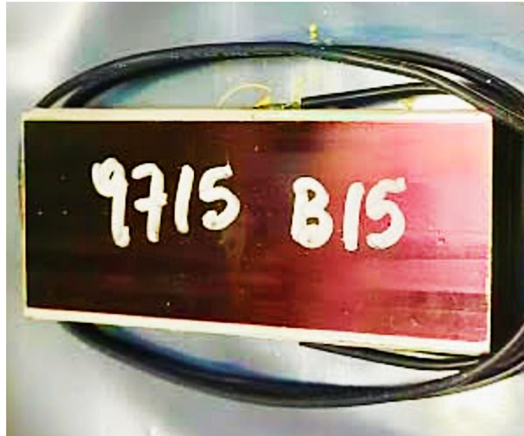
Pulse Capacitor for a Medical Application 140\mu\text{F}/2200 Energy Density: 6.3 \text{ J/cc}
